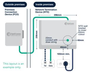
**Indoor installation only.** Opticomm equipment must be installed in a weather protected location such as an enclosed garage or other location allowed under the cabling provider rules.
